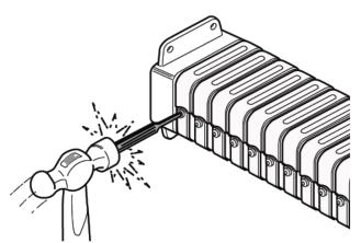
To shorten or lengthen PowerFlex, use a 3/32" punch to drive posts out of rivets securing mounting bracket (above) or links (below). Add or remove links as required. Insert new drive rivets and seat post with hammer as shown in lower left illustration. To repair damaged PowerFlex, remove damaged links and replace. Repairs can be easily made without removing and restringing cables or hoses because nylon inner liners in repair kits are split.
