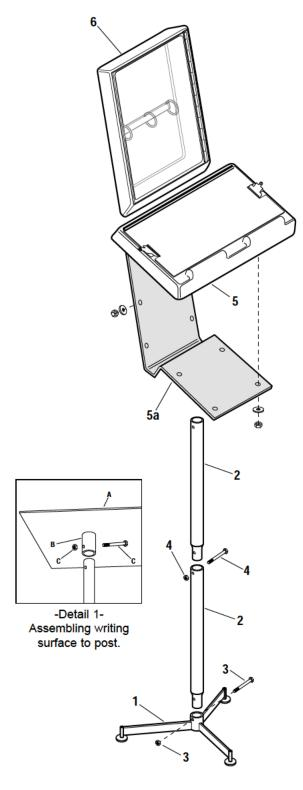
**NOTE:** This stand may be assembled with writing surface (item 5) at a height suitable for either standing use or seated use. To assemble for seated use, substitute 11" long post section for 22 1/2" long section (item 2).
