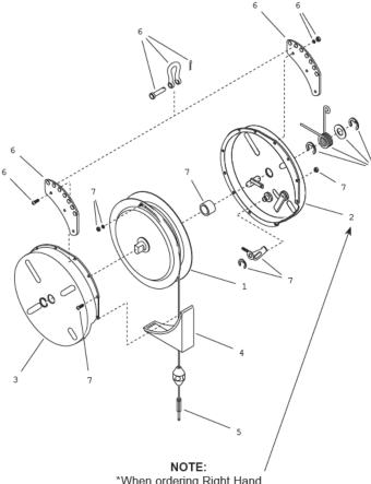
\*When ordering Right Hand Housing Assembly (REF NO. 2) for LOCKING MODELS, you must add "-L" to the kit number.
